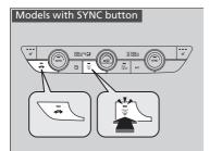
Pressing the (windshield defroster) button turns the air conditioning system on and automatically switches the system to fresh air mode.
