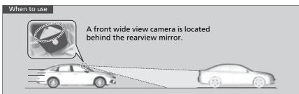
The system starts monitoring the roadway ahead when your vehicle speed is about 3 mph (5 km/h) and will search for a vehicle, pedestrian, or moving bicycle in front of you.
