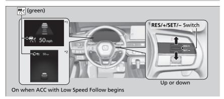
When driving at about 25 mph (40 km/h) or above: Take your foot off the pedal and press the RES/+/SET/– switch up or down when you reach the desired speed. The moment you release the switch, the set speed is fixed, and ACC with Low Speed Follow begins.
