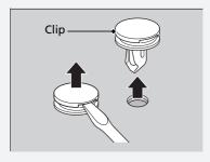
Insert the clip with the pin raised, and push until it is flat.
