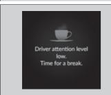
If one bar lights up, the **Driver attention level low. Time for a break.** message will appear, a beep will sound, and the steering wheel will vibrate.
