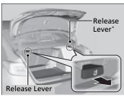
**1.** Pull the release lever in the trunk to release the lock.
