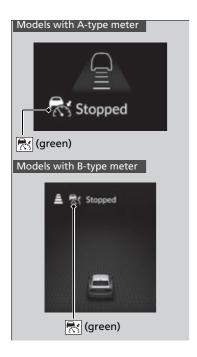
If no vehicle is ahead of you before you resume driving, depress the accelerator pedal and ACC with Low Speed Follow will operate again within the prior set speed.
