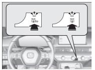
The rear defogger and heated door mirror\* automatically switches off after 10-30 minutes depending on the outside temperature.
