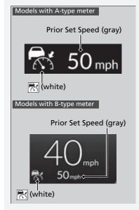
The set speed cannot be set or resumed when ACC with Low Speed Follow has been turned off using the button. Press the system, then set the desired speed.
