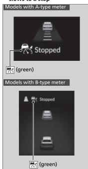
Your vehicle also stops, automatically. The **Stopped** message appears on the gauge. When the vehicle ahead of you starts again, the vehicle icon on the gauge blinks. If you press the **RES/+/SET/-** switch up or down, or depress the accelerator pedal, ACC with Low Speed Follow operates again within the prior set speed.
