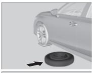
**6.** Place the compact spare tire (wheel side up) under the vehicle body, near the tire that needs to be replaced.
