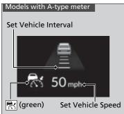
When ACC with Low Speed Follow starts operating, the vehicle icon, interval bars and set speed appear on the gauge.
