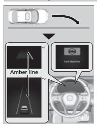
The front camera behind the rearview mirror monitors left and right lane markings in white or yellow, the outer edge of the pavement (bordered by grass or gravel) or a detected oncoming vehicles.
