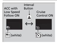
Press and hold the Interval button for one second. **Cruise mode selected** appears on the driver information interface for two seconds, and then the mode switches to Cruise.
