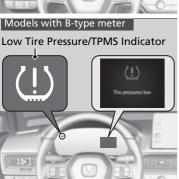
This will cause the low tire pressure/TPMS indicator to come on and a message to appear on the gauge.
