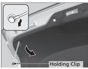
**1.** Remove the holding clip using a flat-tip screwdriver, then pull the lining back.
