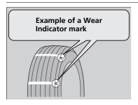
The groove where the wear indicator is located is about 1/16 inch (about 1.6 mm) shallower than elsewhere on the tire. If the tread has worn so that the indicator is exposed, replace the tire. **Worn out tires have poor traction on wet roads.**
