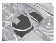
The condition of the battery is monitored by a sensor located on the negative terminal of the battery. If there is a problem with this sensor, the driver information interface will display a warning message. If this happens, have your vehicle inspected by a dealer.
