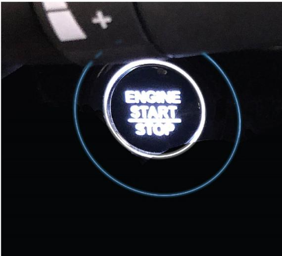
3. Start the engine by pressing the ENGINE START/STOP button while applying the brake pedal. You must start the engine within **10 seconds** of touching the remote to the button.
