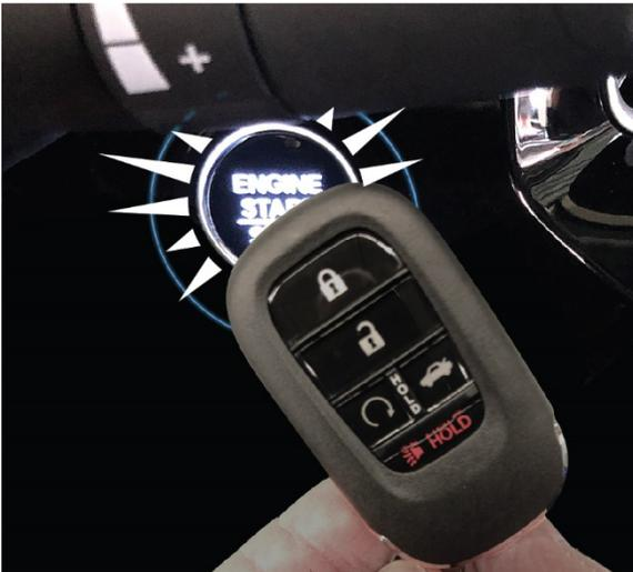
The indicator will switch from blinking to steady when communication is complete.
