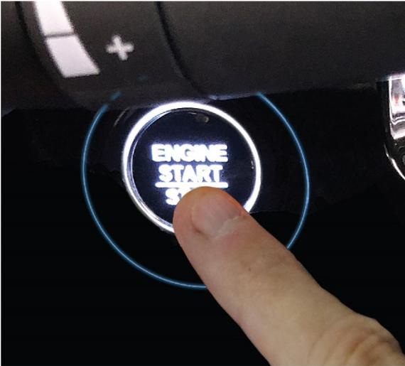
2. Touch the keyless remote to the ENGINE START/STOP button.
