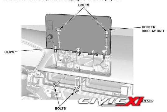
4. Apply 5 x 10 x 1 mm pieces of felt tape as shown in the location shown on both sides, then install the center display unit.
