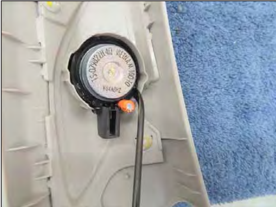
2. Pry out tweeter to release three (3) tabs, then remove tweeter.
