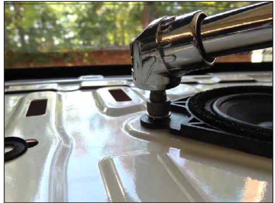
15. Remove two (2) 8mm screws securing speaker to rear deck steel, disconnect harness from inside trunk, then remove speaker.
