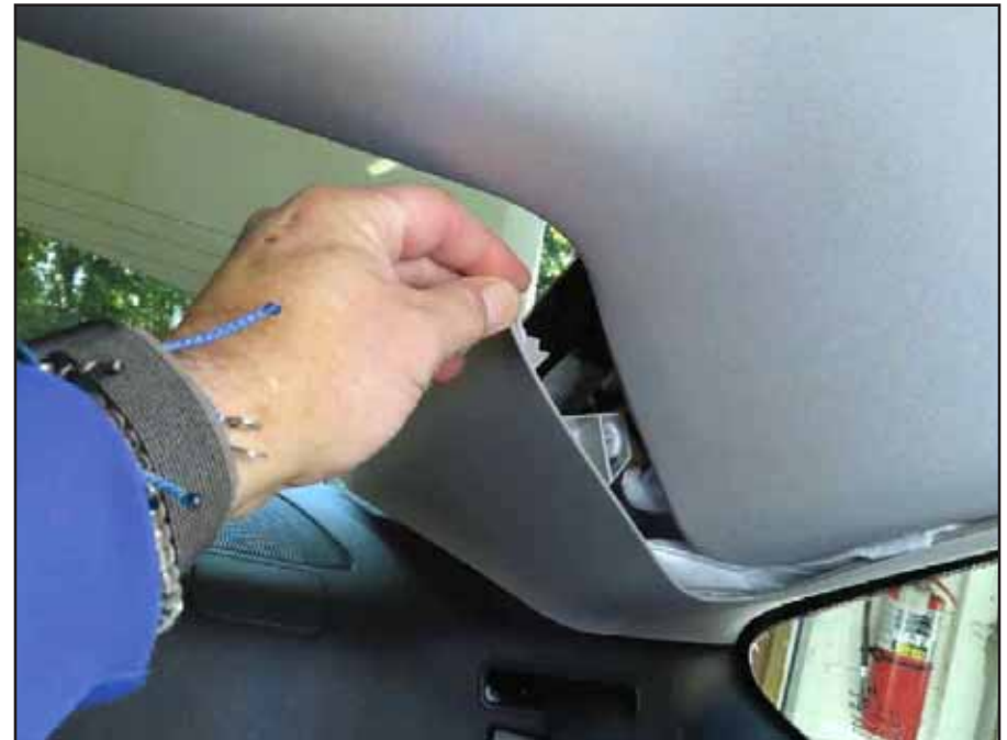
9. Pry off rear pillar trim panel to release seven (7) clips, then pull panel up to remove.
