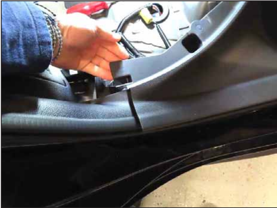
7. Temporarily left up rear seat back cushion, then pry up rear door scuff plate to release seven (7) clips and remove scuff plate.
