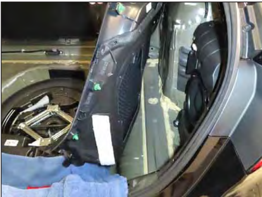
13. Pry out top and side edges of rear side panel to release clips, disconnect harness, then remove side panel.
