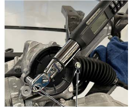
TORQUE BOLTS 8 N·m (6 lb-ft)
