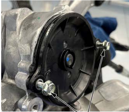
BOLTS Loosely install.
