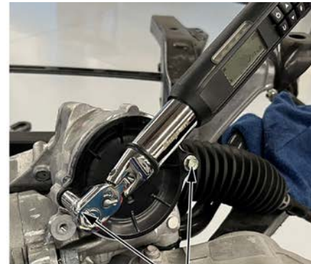
TORQUE BOLTS 8 N·m (6 lb-ft)
