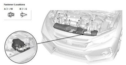
Remove the Hood Seal by undoing 5x Push Clips (A, C) and 6x Push Pins (B).
