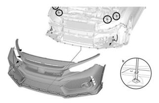
5. Pull the front bumper at the wheel arch area to release it from retaining hooks (B).
