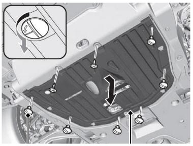
3. Remove the Plastic Undercover that is held down by 3x Push Clips (A), 2x 5mm Socket Head Bolts (B) and 2x Phillips Head Screws (C).
