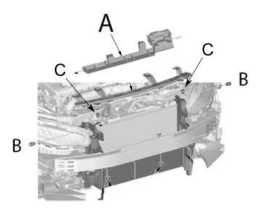
2. Modify the Upper Induction Plate by cutting the plastic as shown here:
