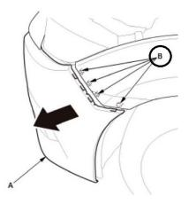
6. Carefully pry on the 3x Retention Hooks under the Headlights (B).
