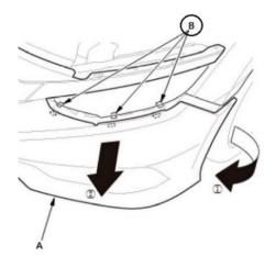
7. Disconnect the Fog Light Harness (a) and remove the Front Bumper.
