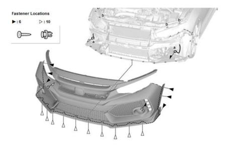
3. Remove 6x Phillips Head Screws and 10x Push Clips.
