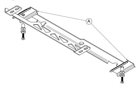
5. Reinstall the Upper Induction Plate and replace any clips that were removed with it previously.
