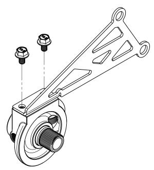
4. Remove the 2x M10 Transmission Case Bolts (A) to install the Pedestal Assembly over the Clutch Line Bracket (C) and using the M10 Washer (B) as a spacer between the Transmission and Pedestal Bracket. Reinstall M10 Transmission Case Bolts and torque to 32lb/ft. (NOTE: Removal of the Upper Clutch Line Bracket Bolt is NOT NECESSARY)
