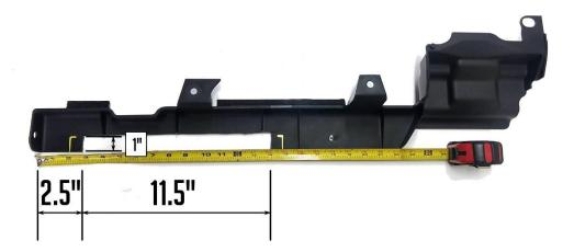
3. Modify the Passenger Side Induction Plate by cutting off the 2x Retaining Grommets that hold it to the bumper beam:
