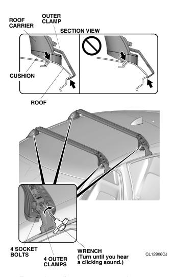
6. Ensure the roof carriers are secured.
